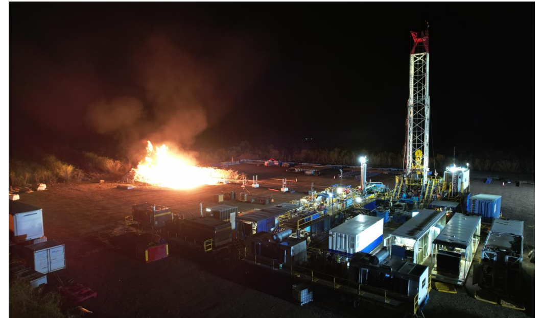
Yandina-5 open-hole flow test @ 7.8MMscfd
